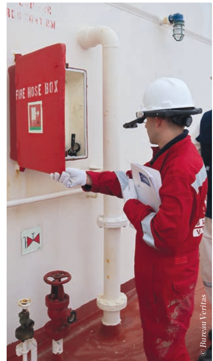
The use of smart glasses on board ships open the possibility to verify and decide remotely, saving time and travel.
